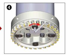
Rotate the adapter's clamping screws clockwise for secure mounting. As you rotate the clamping screw, the clamp will automatically rotate to the locking position.
