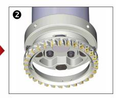
Mount the cutter to the adapter. Check to ensure positioning of the key and key home.
