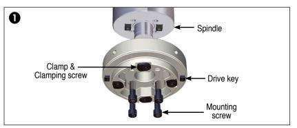
Firmly mount the adapter to the spindle/basic arbor by locking the mounting screws.
