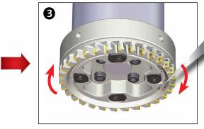
Rotate the cutter as indicated on the cutter face to firmly lock it.
