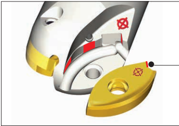
Axial supporting side for stable clamping
