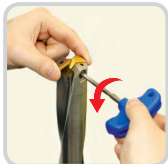
To unclamp, rotate the screw 3-5 times counter-clockwise
